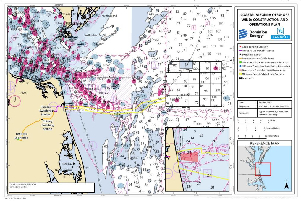
Figure 1-1 Coastal Virginia Offshore Wind Commercial Lease Area (OCS-A-0483) And Planned Export Cable Corridor
